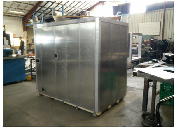
Assembled offshore enclosure 组装好的海工用隔音罩
