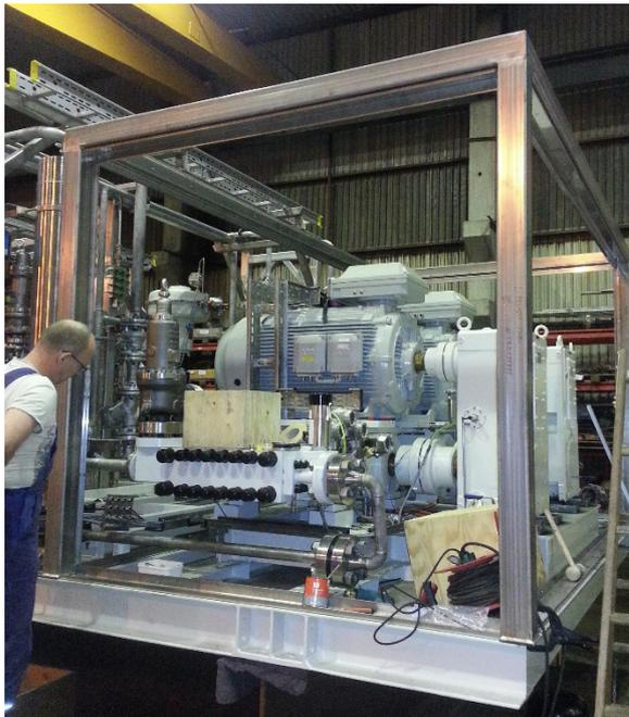
Heavy duty Frame for enclosure panels
